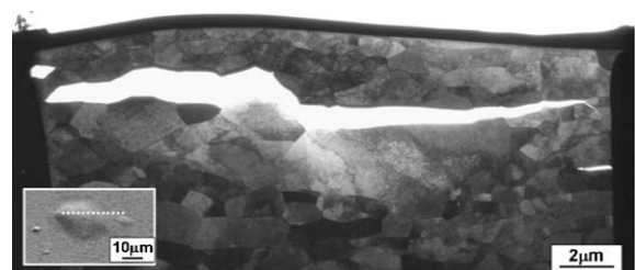
Fig. 3. Cross-sectional TEM image of large blister at the case of (1) + (2) fabricated by FIB technique.
